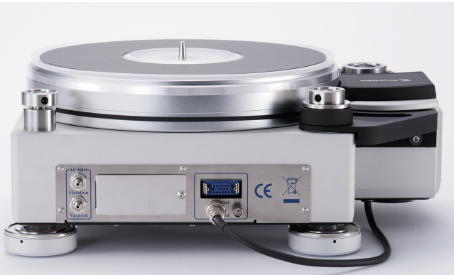
The rear panel is equipped with ‘Flotation’ and ‘Vacuum’ terminals that connect to the power supply unit (other configurations may vary depending on shipment). The drive belt adopts the same 4mm-wide flat belt used in higher-end models.
