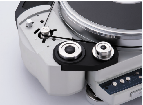
The drive motor unit, separated from the chassis, features the same low-vibration two-phase, four-pole AC synchronous motor used in higher-end models. Its power supply utilizes digitally controlled rotation driven by power amplifiers.
